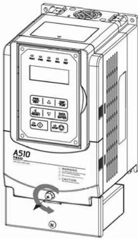
Step 1: Loose screws
