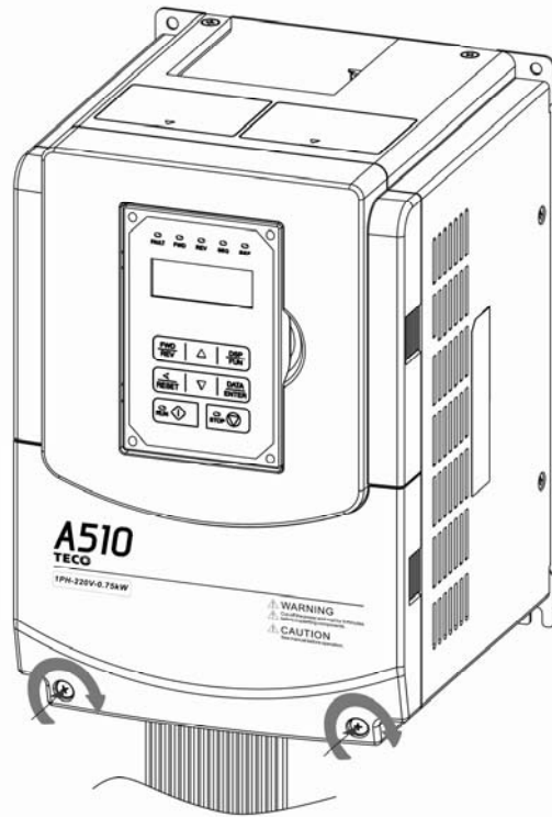
Step 4: Fasten screws
