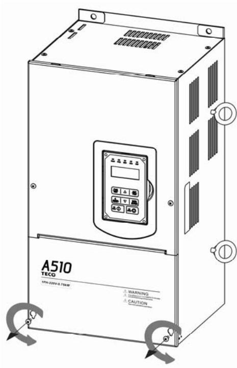
Step 1: Loose screws
