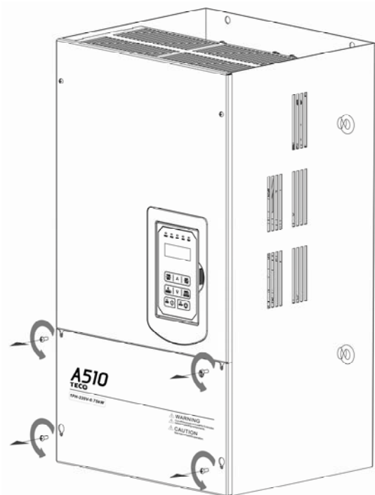
Step 1: Loose screws
