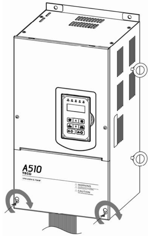
Step 4: Fasten screws
