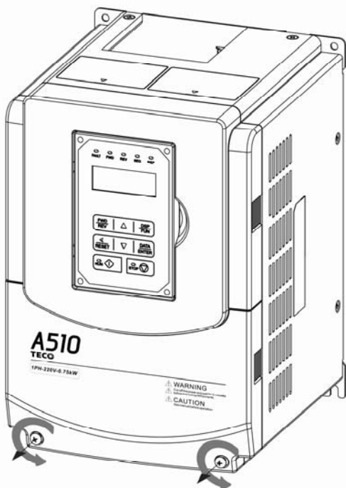
Step 1: Loose screws
